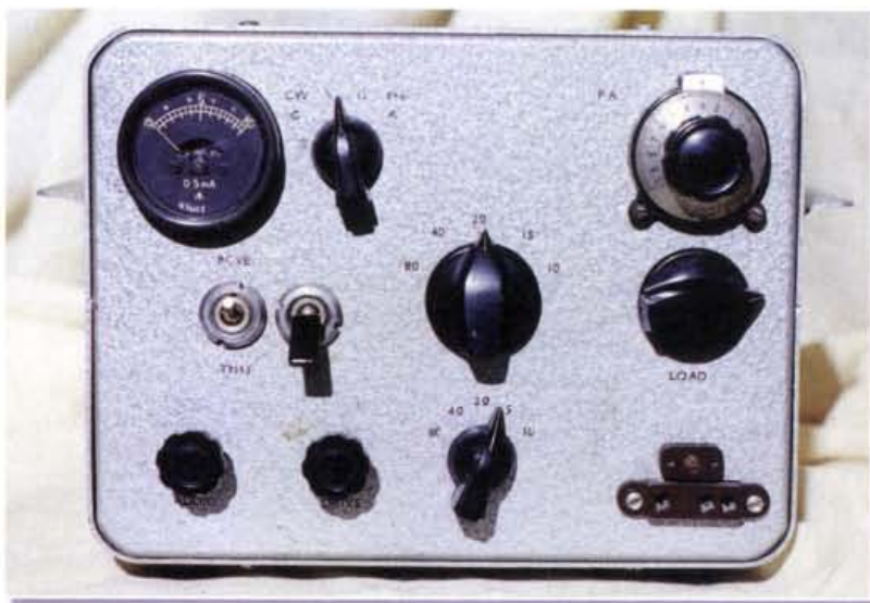
Fig. 2: The little 'home-brewed' transmitter found by G4BXD at the Castle Donington show. Using a crystal-controlled oscillator it provides a good 10W output from 3.5 to 28MHz (see text).
