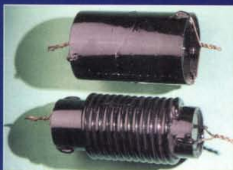
Two variation of 7MHz tuned traps, one internally coiled and one still on the original former. With these versions extra care is needed to ensure that they are fully sealed from the weather.
