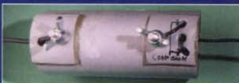
Showing the strain relief holes in operation with the wire forming the elements.
