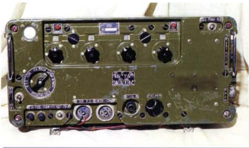
Fig. 3: The Chinese Type 889 transceiver, the operating frequency is selected by the four knobs along the top. A meter (top left) measures all the set's various voltages (using the selector knob directly below the meter).
