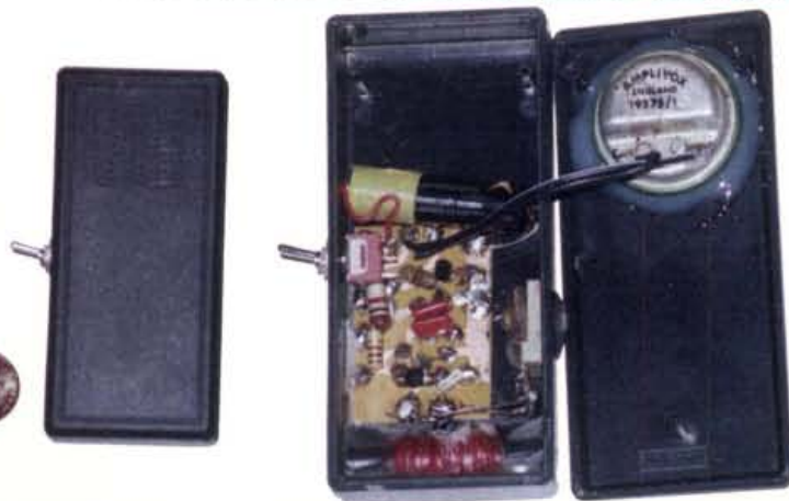
Fig. 9: A single band (long wave) fixed tuned 198kHz BBC Radio 4 receiver built by G3XFD using the MK484 and BC184 combination and an integrally-mounted earpiece. Note the pile-wound ferrite rod antenna - sealed in wax (at the bottom of picture) the 'postage stamp' tuning trimmer and that the sealed (using epoxy resin adhesive) in earpiece and battery, both of which are as far from the antenna as possible for good reception.
