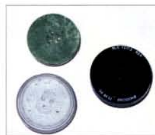
Fig. 2: A selection of the various types of telephone earpiece inserts available as 'surplus'. Offering a relatively low impedance these units are remarkable sensitive and robust and are very useful for use in radio projects (see text).
