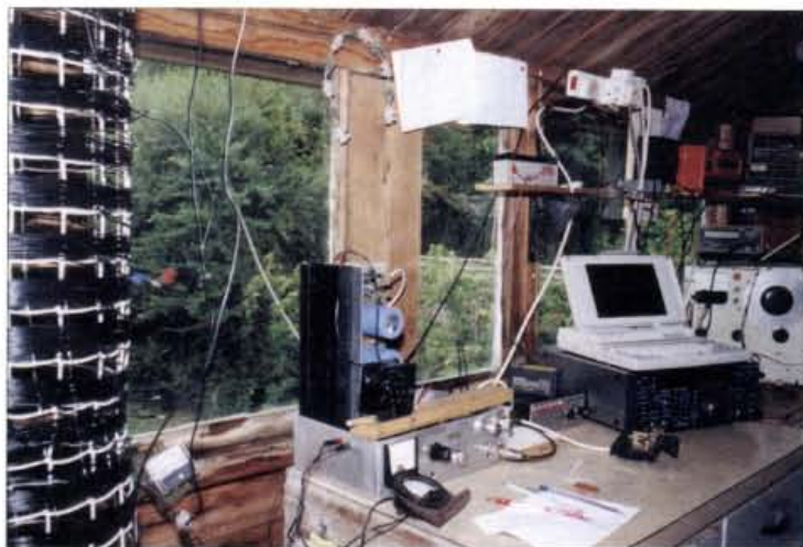
The 136kHz station operated by G3LDO - note that the computer (right) can play a major part in the low power DX QSOs on this band as the signals can often appear to be 'buried' under the noise.
