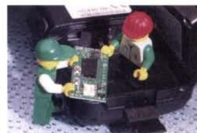
Fig. 2: The SU-1 Barometric Adapter comes as a tiny p.c.b. (compare with Lego man!) which then allows the VX-5R to measure (and show) both 'Altitude' and 'Barometric Pressure'. Yaesu do say, though, that these measurements aren't to be used in the course of any activity where the information is depended on for safety reasons.
