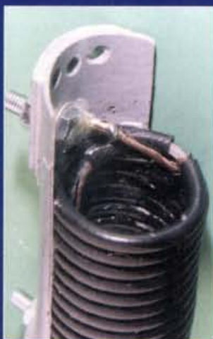
Detail of the end where the coaxial braid is connected to the element. Note the piece of outer insulation used to cover the join of the inner conductor to the short length of heavy copper wire, and the strain relief holes in the 'top' lip.
