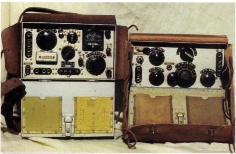
Fig. 4: The Japanese h.f. transmitter (left) and receiver (right). The various multiple pin sockets are for power and signal connections between units. The two-pin socket (bottom left on the transmitter unit) is the 'jack' for the telegraphy key.
