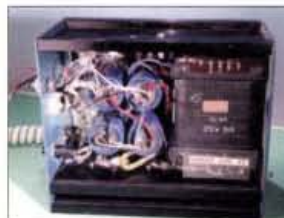
Fig. 11: My own '12V' p.s.u., now many years since I rewired it, but still going strong supplying 10A continuous and up to 15A peak without problems. Note all components are conservatively rated and so, run quite cool, even at maximum loading.
