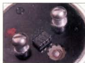
Fig. 10: A close up view of the very heavyweight terminals of the good smoothing capacitor with an 8-pin i.c. for size comparison. The rubber seal near the i.c. is a 'gassing' indicator, showing if the capacitor has been subject to some over-voltage or over-current abuse and may be damaged.
