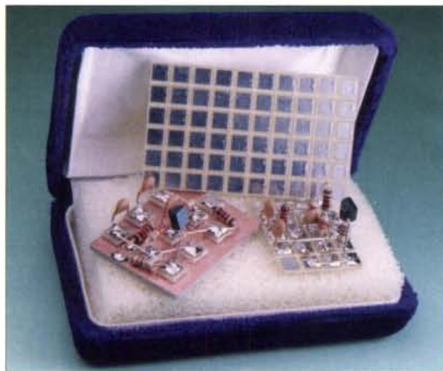
'Lifting the lid' on some of the methods employed with 'Ugly' construction and using printed circuit board material for non-printed circuit design.
