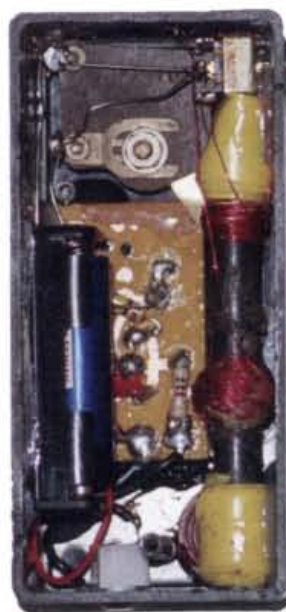
Fig. 10: A two band MK484 receiver (no extra amplifier) employing a Jackson solid dielectric 500pF tuning capacitor and 'shock mounted' ferrite rod assembly (see text). This receiver uses a separate earpiece and was built by G3XFD for his own use.
