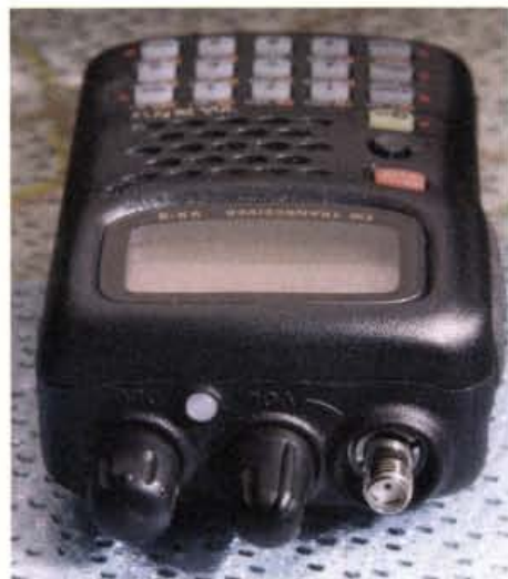
Fig. 4: Top of the VX-5R. You attach the helical antenna on the right. The control in the middle is the volume (VOL) and on the far left is the 'DIAL' control.
